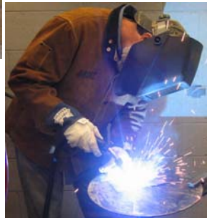
Flux Cored electrode Welding (FCW)
