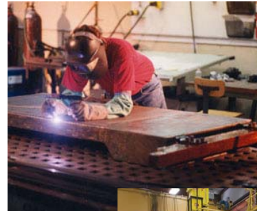
Metal Inert Gas (MIG): solid metal wire may contain Ni
